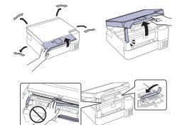
To close the scanner unit, lift the scanner unit slightly, then lower it until it stops. Repeat the motion to fully close the scanner unit.
