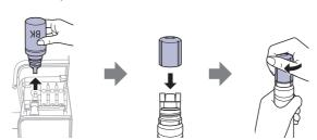
Note: Do not leave the ink bottle inserted; otherwise the bottle may be damaged or ink may leak. If any ink remains in the bottle, store the bottle upright and top off the ink tank after completing initial setup.
