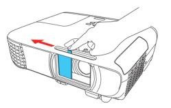
Press the opening power button on the projector or remote control. The projector beeps, the Status light flashes blue, and then stays on.
