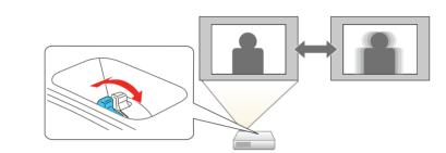
If your image looks like or , you may have placed the projector off to one side of the screen at an angle. Place the projector directly in front of the center of the screen, facing the screen squarely. If you can't move the projector, use the horizontal keystone slider on the projector to correct the image shape.
