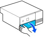
Place your hand as shown in the illustration, 4 and pull out the interior of the printer until it stops.
