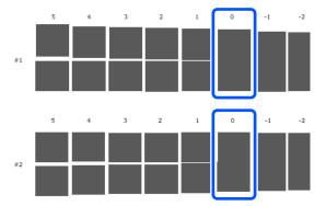
If all of the adjustment patterns contain overlaps or gaps, and you cannot narrow it down to one, select the pattern with the least overlap or gap.
