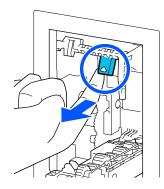
(3) Keep the lever in step 12-(2) raised as you raise the Roller Assembly Kit so that the tips of the protrusions extend out of the holes in the Roller Assembly Kit as shown in the illustration, and then release your finger from the roller lock lever.
