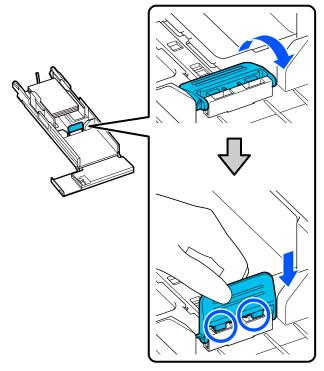
Align the front edge guide to the position of the size of paper to be loaded.
