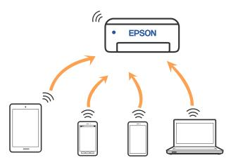
The printer can be connected by wireless LAN (Wi-Fi) and Wi-Fi Direct (Simple AP) simultaneously. However, if you start setting Wi-Fi Direct (Simple AP) while connected by wireless LAN (Wi-Fi), the wireless LAN (Wi-Fi) connection is temporarily disconnected.
