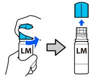
Align the bottle with the ink inlet and insert it, 7 and then wait until the ink stops by itself at the upper limit line (a).
