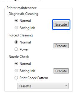
The nozzle check starts and cleaning is executed if necessary.
