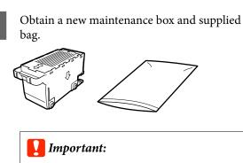
Do not touch the chip on the maintenance box. Doing so may prevent normal operation and printing.
