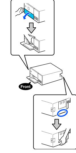
Do not lift the product while its internal components are pulled out. Dropping it could cause an injury.
