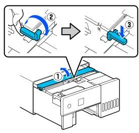
7 Close the inner cover, return the interior of the printer to its original position.
