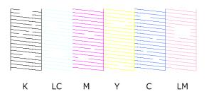
If part of the pattern is missing, then the print head nozzles are clogged. The print head needs to be cleaned.
