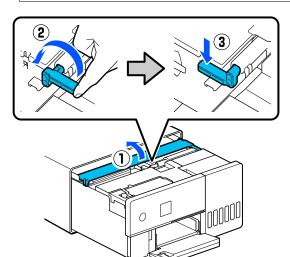
5 Close the inner cover, return the interior of the printer to its original position, and then close the front cover.
