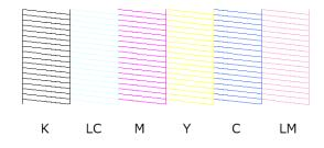
If none of the check pattern is missing, then the print head nozzles are not clogged.
