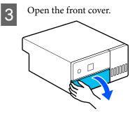
Place your hand as shown in the illustration, and pull out the interior of the printer until it stops.
