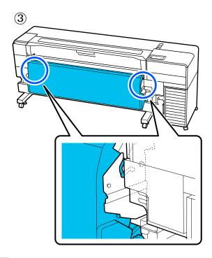
Use the screws that you removed to secure the after heater at the points shown in the illustration on the left and right.
