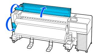
While holding the tabs of the media edge plate you want to replace on both sides, move the plate to the left edge of the platen heater to remove it.
