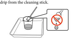
When soaking a clean-room wiper with ink cleaner, use the ink cleaner poured into the container.
