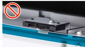
Hold the carriage scale to bend the part with the hole, as shown in the illustration, and insert it from below into the left and right tabs of the scale holder.
