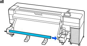
Insert the left media holder into the roll core and press it against the roll core twice.
