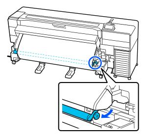
Check that the media is installed without any warping.
