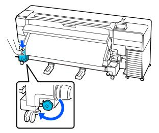
Turn the handle until the part labeled A in the following illustration is fully inserted.
