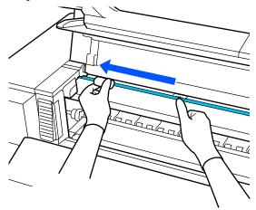
Switch the hand pressing it down, and wipe 10 times from the scale holder to the right.
