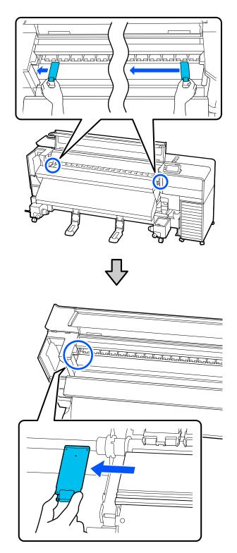
Insert a new media edge plate into the left edge of the platen heater.
