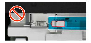
If it has detached, gently pull the carriage scale to the right and hook the hole over the hook.
