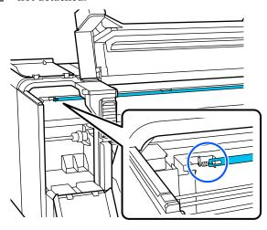
The carriage scale has detached if the hole in the scale extends in front of the hook.
