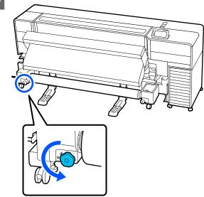
While supporting the media from below with your hand to prevent it from falling, pull out the media holder and lower the media onto the media supports.
