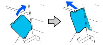
When using the auto take-up reel unit, store the tension bar.
