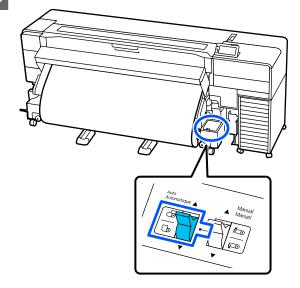
Position the Manual switch based on the take-up direction and take-up specifications to take-up the media around the roll core for one complete turn.
