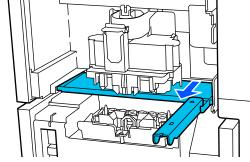
Position the lever with the ▲ mark facing up, and store the lever.
