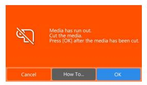
Open the printer cover and remove the roll core of the finished media and the rewound media while checking the procedure on the panel's screen.
