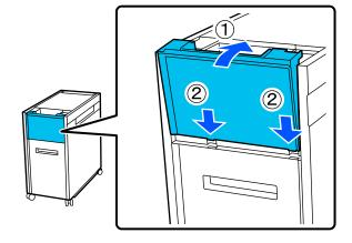
Make sure you remove the ink tube connector cover before moving.
