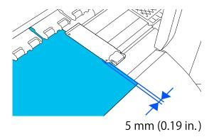
The edges of the media are not detected correctly if the media edge plates are not attached correctly.
