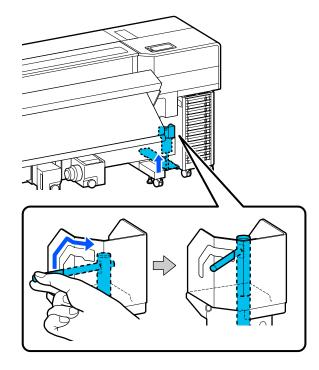
Unlock the casters on the bulk ink solution.
