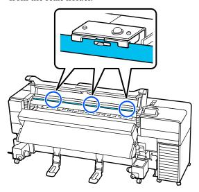
It has not detached if the left and right tabs of the scale holder and the protruding part at the center of the holder extend beyond the scale. If it has detached, follow the steps below to reattach it.
