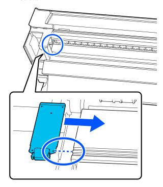
Check that two hooked sections at the rear of the media edge plate are securely applied as shown below and that they are attached with no gap between the platen heater and media edge plate.
