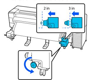
While pressing down on the media holder, securely tighten the locking screw.
