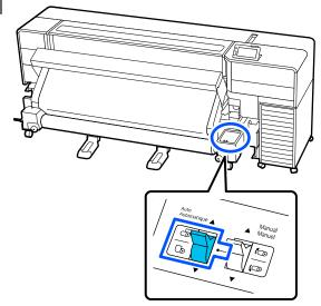
Take up the cut media completely by positioning the Manual switch according to how the media is rolled.
