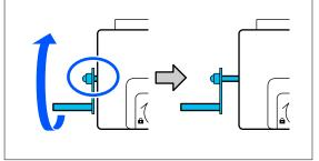
Loosen the locking screw on the right media holder and move it to the loading position that matches the inner diameter of the roll core.
