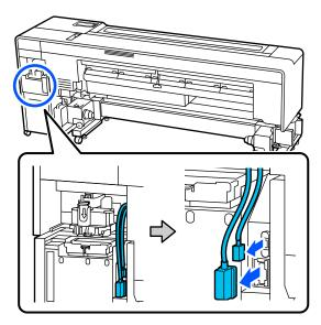
Remove the lever from the bulk ink solution.
