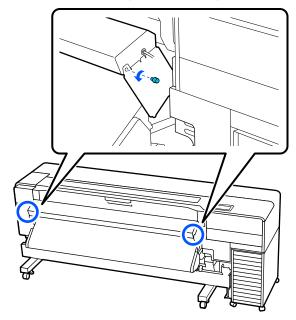
Grip the sides and pull the drying fan straight up to remove it.
