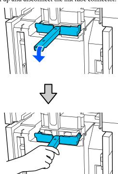
Hold the knob for the ink tube connector, then lift the connector and secure it at the top.
