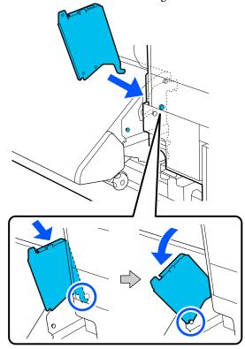
☐ Install the drying fan by inserting the left and right hooks into the holes shown in the illustration and then sliding it slightly toward you.
