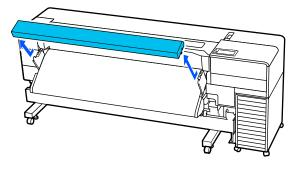
Remove the screws shown in the illustration from the left and right drying fan installation plates.
