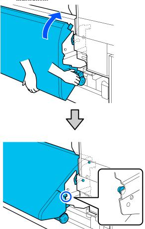
☐ Install the drying fan installation plates by inserting the tip at the position shown in the illustration and then lowering it down.
