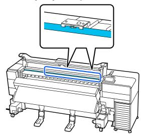
Check that the carriage scale has not detached from the scale holder.
