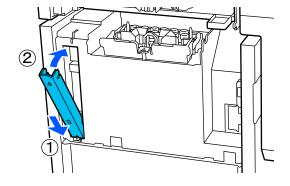
Go to the front of the printer and lift up the securing section of the bulk ink solution to release it.
