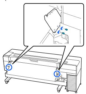
Remove the drying fan installation plates.
