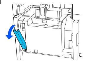
Pull the lock handle toward you, and insert the notch at the end of the lever onto the lock handle.
