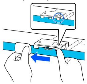
Repeat steps 5 to 7 for the remaining two locations to wipe the entire carriage scale.
