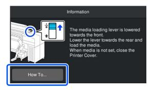
On the How To screen, press the button shown in the illustration to rotate the display 180°. Tilt the control panel and rotate the display for easier viewing when working at the back of the printer.
