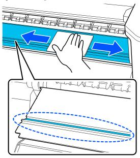
Soak a soft cloth in water, wring it out thoroughly, and then wipe off any lint, or dust that has adhered to the media edge plates.
