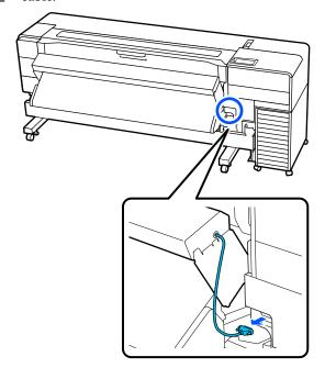
Remove the screws shown in the illustration from the left and right of the drying fan.
