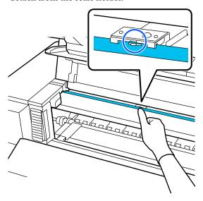
While pressing the scale holder, use a clean-room wiper to grip the carriage scale and wipe off ink stains from the front and back surfaces of the scale.
