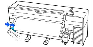
While pressing down on the media holder, securely tighten the locking screw.
