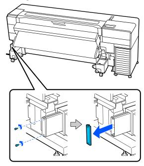
Loosen the locking screws on the media holders and remove them both.
