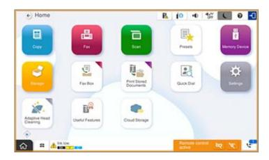
This is the screen displayed when you make settings in Web Config to prevent the user from disconnecting the remote connection or hiding the remote screen using the printer's operation panel. The remote control menu is not displayed at the bottom right.
