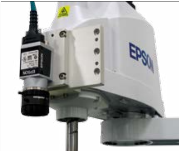
T3 shown with mobile mounted camera as a part of the Epson Vision Guide option
