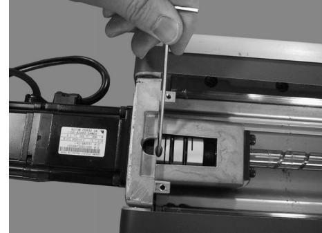
(5) Mount the stop in the module body and secure the stop with the two hexagon socket head cap bolts (M4×10).
