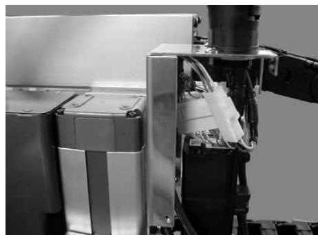
Put the wire tie through two holes on the U support 2 and fasten the cables with the wire tie.
