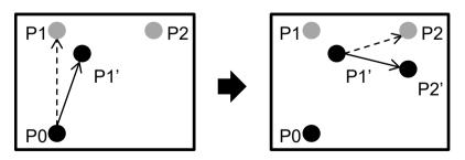
In the first Move, a trajectory from the initial position P0 to the target position P1 is planned (dotted line), and then the robot starts motion.
