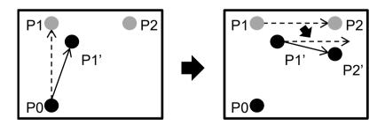
In the first Move, a trajectory from the initial position P0 to the target position P1 is planned (dotted line), and then the robot starts motion.
