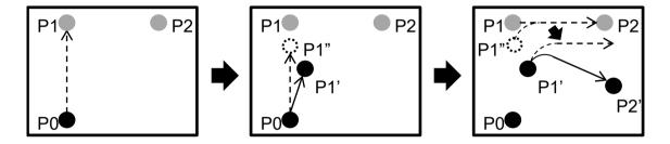
In the first Move, a trajectory from the initial position P0 to the target position P1 is planned (dashed line), and then the robot starts motion.
