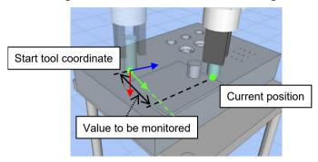
The orientation will be determined either by the angle between the axis (X, Y, or Z) specified by the Rot\_Axes property in the current tool coordinate system and the axis in the tool coordinate system at the start of monitoring, or by the amount of rotation of arbitrary axis. If X is the specified axis, this will determine the angle between the X axis at the start of monitoring, and the current X axis as shown in the diagram below.
