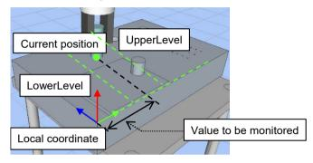
The orientation will be determined either by the angle between the base coordinate system or the local coordinate system used as the basis for robot positions and the axis (X, Y, or Z) specified by the Rot\_Axes property in the tool coordinate system, or by the amount of rotation of arbitrary axis. If X is the specified axis, this will determine the angle between the X axis in the reference coordinate system and the X axis in the current tool coordinate system as shown in the diagram below.
