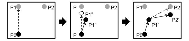
In the first Move, a trajectory from the initial position P0 to the target position P1 is planned (dotted line), and then the robot starts motion.
