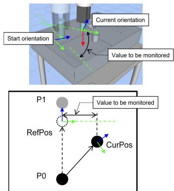
The orientation will be determined either by the angle between the axes (X, Y, or Z) specified by the Rot\_Axes property in RefPos and CurPos, or by the amount of rotation of arbitrary axis
