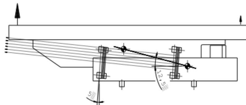
Spring angle is smaller than the gravity center angle
