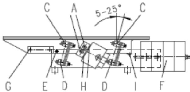
Unscrew the 4 or 6 upper lateral spring fastening screws (“C”) (M6 DIN 912). The complete oscillator with mounted track can now be lifted upwards. Remove the desired spring pack by releasing the lower lateral spring fastening screws (“D”) (M6 DIN 912).
