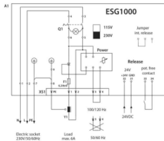
The jumper must be diverted to enable the external release.
