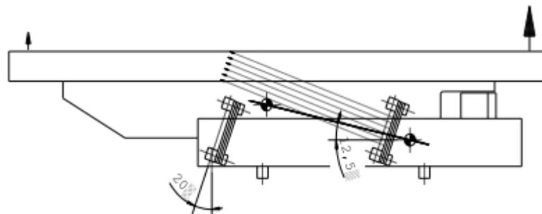
Spring angle larger than the gravity center angle
