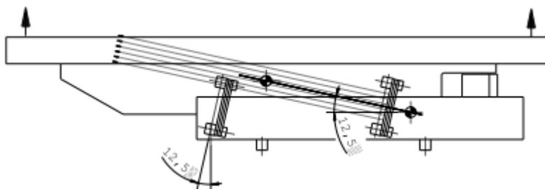
Spring angle equals gravity center angle
