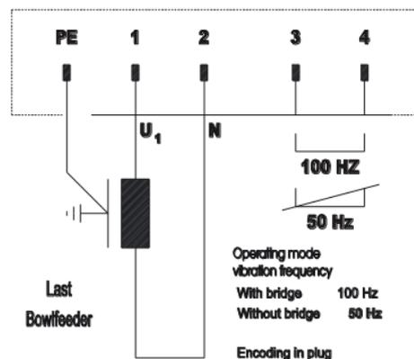
With bridge: The bridge has to be installed in connection 3 + 4
