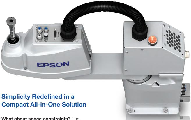
The Synthis T3 All-in-One SCARA robot with built-in controller provides fast integration at an ultra low cost
