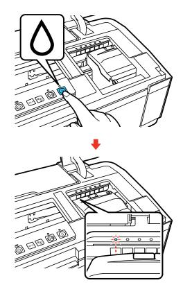
**Note:** If an ink cartridge is low, a flashing light appears above it. You can continue to use the low ink cartridge until it is expended. Do not hold the  $\Diamond$  ink button for more than three seconds, or the product may start cleaning the print head.
