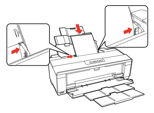
**Note:** During printing the left edge guide automatically moves 0.12 inch (3 mm) to the left. Do not move it back manually.
