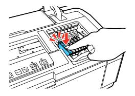
9. Once you replace all the cartridges that need replacing, close the cartridge cover and the printer cover.
