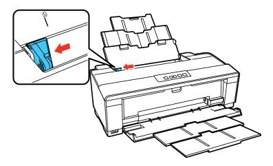
4. Insert paper, glossy or printable side up and short edge first, against the right side and behind the tab. Then, slide the edge guide against the paper, but not too tightly. If you are inserting a stack of paper, fan the sheets first and tap the stack on a flat surface to even the edges.
