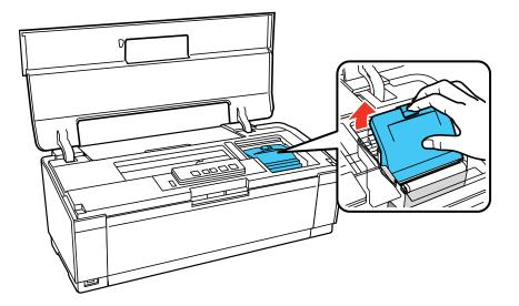
5. Squeeze the tab on the cartridge and lift the cartridge straight up to remove it.
