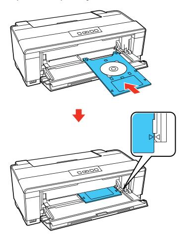
**Caution:** Do not insert the CD/DVD tray while the <sup>(b)</sup> power light is flashing. Otherwise, the product or your CD/DVD may be damaged. Do not turn off the product with the CD/DVD tray inserted in it. Always remove the tray first.
