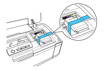
**Note:** Some tape may be difficult to remove if left in place for a long time. Remove the tape immediately after transporting the product.
