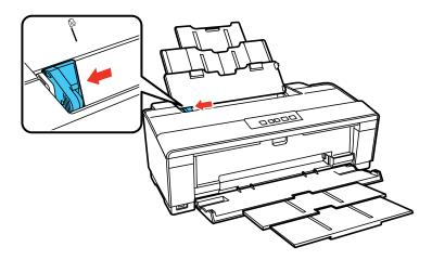
4. Load up to 10 envelopes against the right side, printable side up, and flap edge left. Then, slide the edge guide against the envelopes, but not too tightly.
