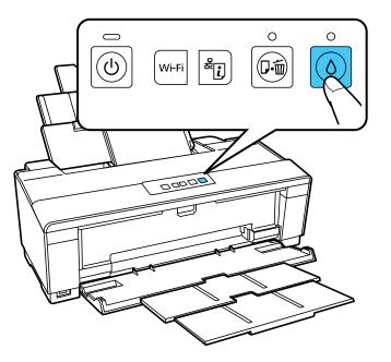
The  $\bigcirc$  power light flashes throughout the cleaning cycle and stays on when the cleaning cycle is finished.
