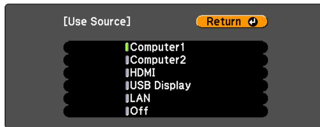
4. Select the source where the computer is connected. For example, if you connected the computer to the projector’s **Computer1** port, select **Computer 1**. If you connected the computer to the projector’s **HDMI** port, select **HDMI**.
