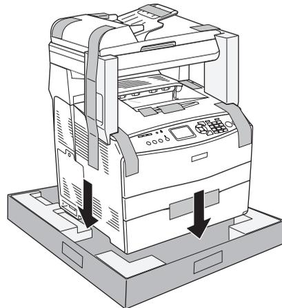
15. Attach foam to the top corners of the CX11N/CX11NF as shown below:
