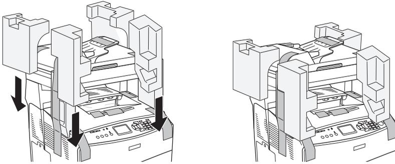
16. Lower the top of the original box and attach the four white handles, turning them to the closed (locked) position. Then tape the top of the box closed with shipping tape.
