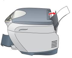
Position the Stylus CX so the front is at least 9 inches from the edge of the table.
