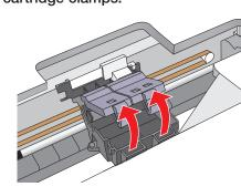
6 Insert the ink cartridges with the labels face-up.
