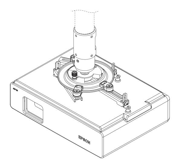
Maximum UL Load Capacity: 50 lb (22.7 kg)
