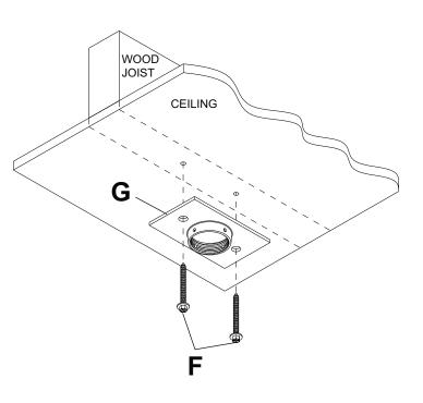
IMPORTANT: Be sure to drill holes into the joist CENTER!
