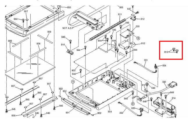
The correct part and reference numbers for the Expression 1600/1680 Transparency Unit (B813182) lock-down thumbscrews are respectively: 1012588 and 815. The Parts Price List (PPL) description is S. THUMB SCREW M4X10 F/NI, Quantity = 2.
