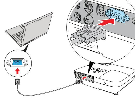
Connect one end to the projector's **Computer (Component Video)** port, and the other end to your computer's monitor port. If you are using a notebook, switch it to external display. You can also connect an audio cable.
