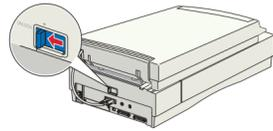
**2** Connect the scanner to your computer using either the USB or FireWire cable that came with your scanner, or a SCSI cable. **Don't connect more than one cable.**
