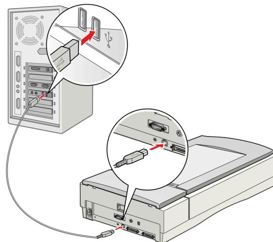
**Note:** Your scanner may not work correctly if you use a USB cable other than the one supplied by EPSON, or if you connect your scanner to a multi-level USB hub system.
