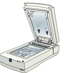
6 Gently close the transparency unit. Connect the transparency unit cable to the **OPTION** connector at the back of the scanner and tighten the screws.
