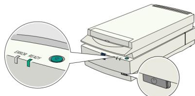
**5** **USB:** When the **READY** light stops flashing, you're ready to scan.
