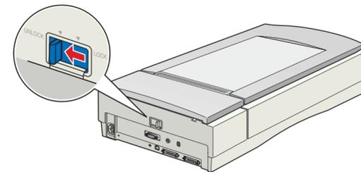
**Caution:** Your scanner won't work unless the transportation lock is in the **UNLOCK** position. Also, you may damage the scanner if you leave it on while it's locked.
