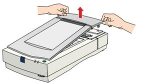
3 Place the transparency unit on a flat surface, glass side up. Remove the tape. Then remove the shipping screw from the hole labeled **CLAMP** and install it in the hole labeled **STOCK**.
