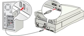
**Note:** Your scanner may not work correctly if you use a USB cable other than the one supplied by EPSON, or if you connect your scanner to a multi-level USB hub system.
