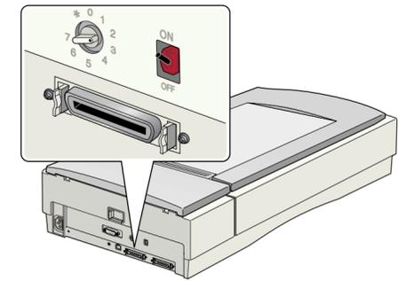
Unless your scanner is connected in the middle of a SCSI chain, leave the terminator switch on the back of the scanner turned **ON**.
