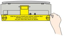
2 Remove the scanner cover by grasping the back of the cover and easing it up.
