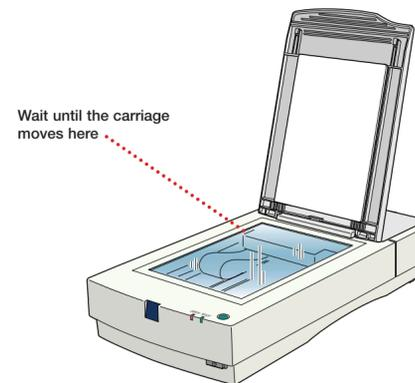
**Note:** If the carriage doesn't return to the home position automatically, slowly raise the front of the scanner and let the carriage slide to the home position.
