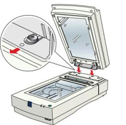
5 Insert the two screws that came with the transparency unit into the screw holes, and tighten them with a coin.
