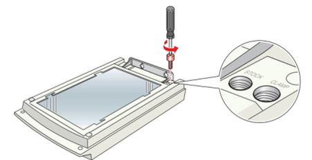
**Caution:** Never use the transparency unit without removing the shipping screw from the hole labeled **CLAMP**. You may damage the unit.
