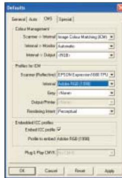
**7** For the **Scanner (Reflective)** or **Scanner (Transparency)** settings, select the Monaco scanner profiles you created. For the **Internal** setting, select **Adobe RGB (1998)**.
