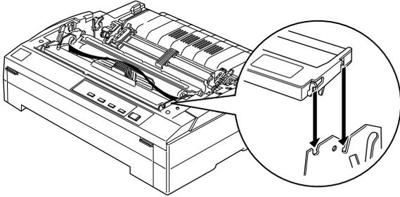
7. Use a pointed object, such as a ball point pen, to guide the ribbon between the print head and ribbon guide while you turn the ribbon-tightening knob to help feed the ribbon into place.
