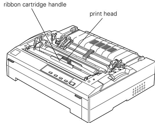
4. Grasp the used ribbon cartridge by its handle and pull it up and out of the printer.
