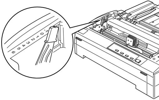
The paper thickness lever is located under the printer cover.
