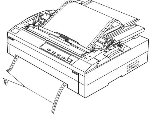
4. Turn the knob on the left side of the printer away from you to eject the paper in the printer.
