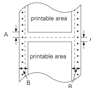
A The minimum top and bottom margins (above and below the perforation) are 0.17 inch (4.2 mm).
