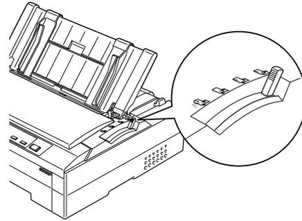
Use the paper release lever to select which paper source you want the printer to load paper from. The table below shows the corresponding paper path(s) for each paper release lever position.
