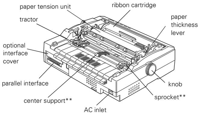
\* The paper guide support frame is beneath the continuous paper support.
