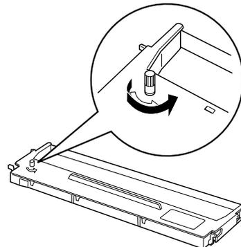
6. Hold the ribbon cartridge by its handle and push it firmly down into position; then press down both ends of the cartridge to fit the plastic hooks into the slots.
