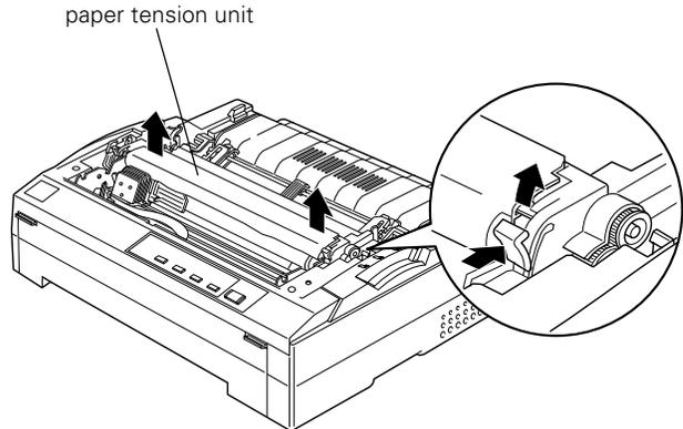
3. Make sure that the print head is not hot; then slide the print head to the middle of the printer by hand.
