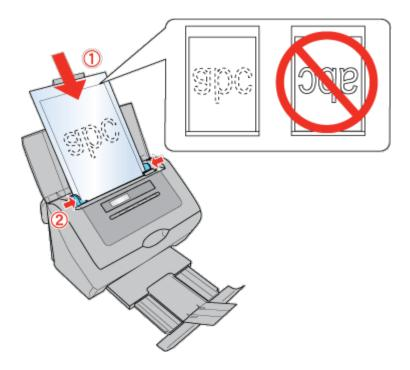
Slide the carrier sheet into the feeder until it meets resistance. Then slide the edge guides over to fit the edges of the carrier sheet.
