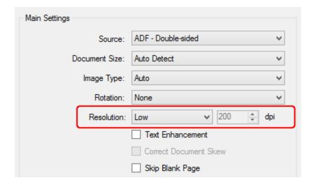
Click the arrow next to the **Resolution** list and select a setting. Select the **Low** setting for 200 dpi (dots per inch), the **Medium** setting for 300 dpi, and the **High** setting for 600 dpi. If you select **Custom**, you can pick the number of dpi at which you want to scan.
