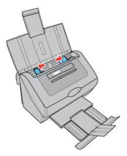
Load your documents into the input tray with the printed side facing down and the top edge facing into the feeder.
