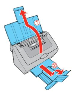
Slide the edge guides on the input tray all the way outward.
