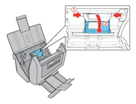
8 Slide and remove the installed paper feed roller.
