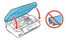
6 Press OK to prime the ink delivery system. Priming takes about 4 minutes.
