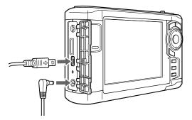
**3** Connect the other end of the cable to the USB connector on the printer.
