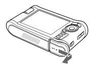
**3** Insert the battery into the compartment in the direction of the arrow on the battery.
