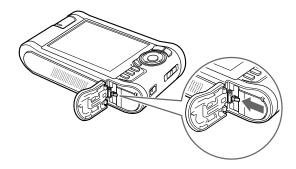
**4** Pull out the battery. Then close the battery cover.
