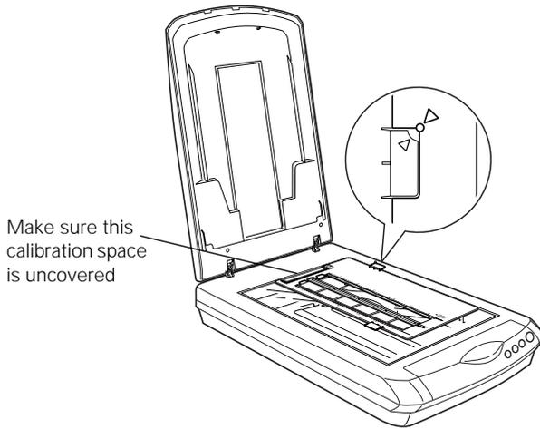
If you are scanning slides, place the holder on the scanner. Then place the slides in the holder. (Place the slides so the "this side to lamp" indication is facing down.)
