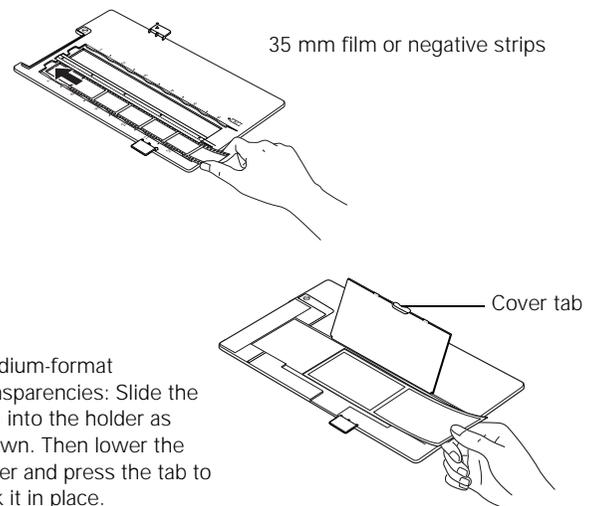
Medium-format transparencies: Slide the film into the holder as shown. Then lower the cover and press the tab to lock it in place.
