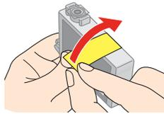
Do not remove or tear the label or other seals on the cartridge; this can cause leakage.
