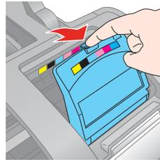
7. Squeeze the tab at the back of the cartridge and lift it straight out. Dispose of it carefully. Don't take the used cartridge apart or try to refill it.
