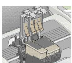
Don't place the cartridge tabs **under** the hooks; you may damage the clamp when you close it.
