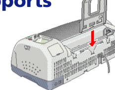
Insert the roll paper adapter into the slots on the back of the printer.
