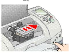
Ink charging takes about two minutes. You will see the lights flash and hear the printer make noise. Don't turn off the printer during this process or you'll waste ink.
