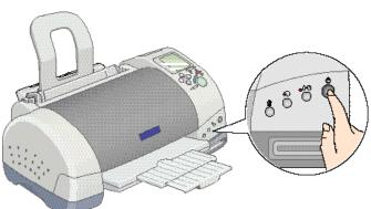
Press the silver  $\bigcirc$  power button to turn on the printer.
