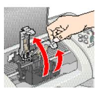
Install both ink cartridges, and leave them installed for all types of printing, or the printer won't work.
