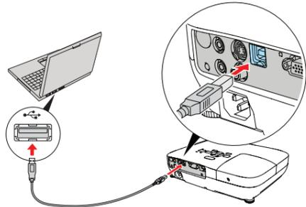
**Windows®:** After turning on the projector, follow the on-screen instructions to install the Epson USB Display software (EMP\_UDSE.EXE; only on first connection).
