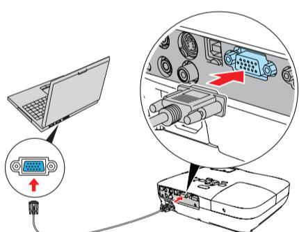
**PowerLite S9:** You can also connect an external monitor to the **Monitor Out** port. See the *User's Guide* on your projector CD.
