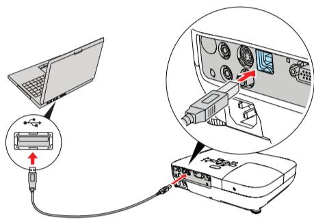
**Windows®:** After turning on the projector, follow the on-screen instructions to install the Epson USB Display software (EMP\_UDSE.EXE; only on first connection).
