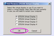
When you click "OK", the drivers for the virtual display are enabled. At this point, it is normal for the display to flicker. Wait for the "Add/Remove Epson Virtual Display" screen to close.
