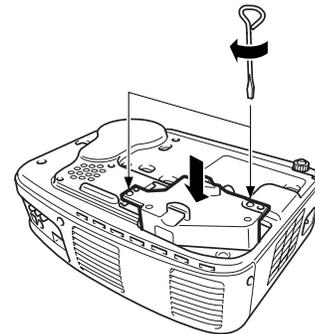
7. Insert the lamp cover as shown and press it back into place.
