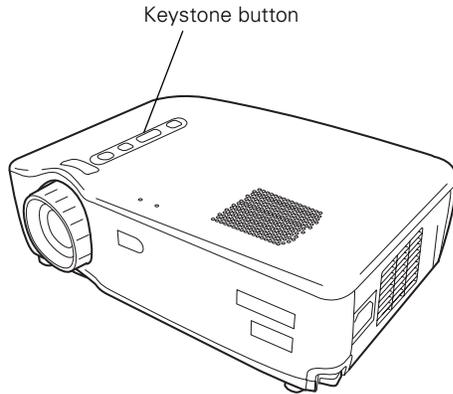
The **Keystone** button corrects up to a 15° tilt. You can also perform electronic keystone correction using the projector's Setting menu.
