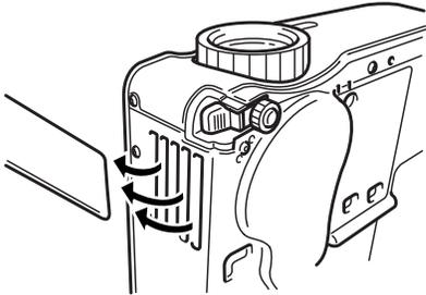
3. To clean the vent, EPSON recommends using a small vacuum cleaner designed for computers and other office equipment. If you don't have one, use a dry, lint-free cloth.
