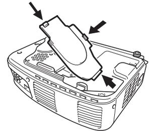
5. Use a screwdriver to loosen the two lamp cover screws; you can't remove the screws. Then pull out the lamp by the two notches.
