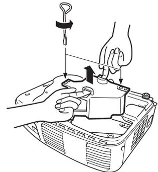
6. Position the new lamp correctly, then gently insert it into the projector. Press it into place and tighten the retaining screws.
