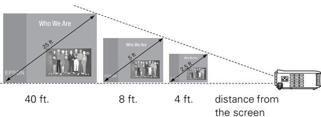
When projecting from a table, the ideal arrangement is to set the projector flat on its surface with the base of the lens at about the level of the bottom of the screen. This delivers the best-looking picture.
