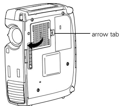
5. To install the new filter, first insert the tabs, then press on the latch until it clicks in place.
