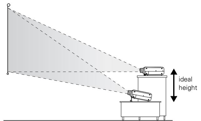
If you place the projector level with the bottom of the screen, the image will be square and you won't have to adjust it. If you place the projector higher than the bottom of the screen, the image will still be square, but you won't be able to fill the whole screen with the image.
