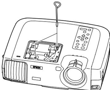
5. Grasp the lamp as shown, and pull the lamp straight out.
