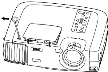
4. Use a screwdriver to loosen the two silver screws holding the lamp in place. (You can't remove these screws.)
