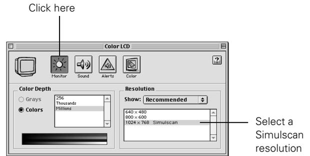
2. Select a Simulscan resolution as shown. Allow a few seconds for the projector to sync up after making the selection.
