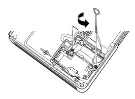
5. Hold the lamp as shown and pull it straight out.
