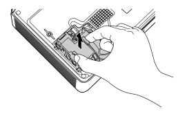
6. Gently insert the new lamp. (If it doesn't fit easily, make sure it is facing the right way.)
