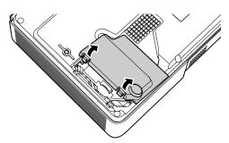
4. Loosen the two screws holding the lamp in place (you don't need to remove them).
