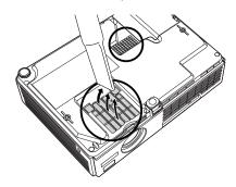
If dirt is difficult to remove or the filter is torn, replace it. The air filter set (part number V13H134A08) contains two filters. Contact your dealer or call Epson at (800) 873-7766 to obtain a new set. In Canada, please call (800) 463-7766 to locate a dealer.
