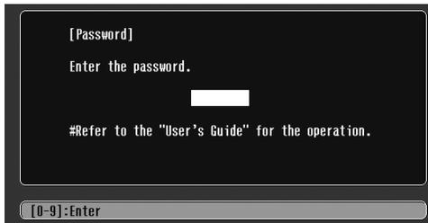
Hold down the Num button on the remote control as you use the numeric keypad to enter the password. Once you enter the password correctly, the screen closes, and projection begins.
