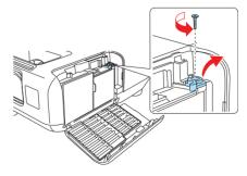
Insert the wireless LAN module into the port.
