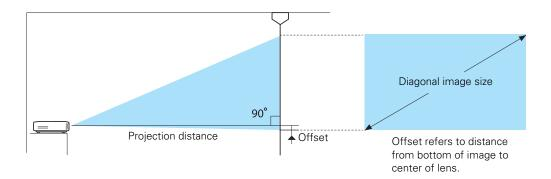
The size of the image is determined by the distance from the projector's lens to the screen. Depending on your display settings and how you use the zoom ring, the actual size may differ. Use these tables as a guide for projector placement:
