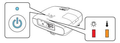
If the projector isn't working correctly, first press the  $\circlearrowleft$  power button, let the projector cool down, and unplug the power cord. Then plug the power cord back in and turn on the projector. If this doesn't solve the problem, check the status lights on top of the projector.
