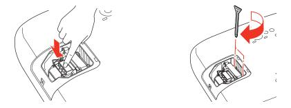
Replace the lamp cover. (The projector won't work if the lamp cover is open or loose.)
