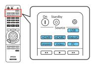
If you press the \( \operatorname{F} \) Source button on the projector, you see a list of available sources. Press the Source button to move through the list and select the desired source.
