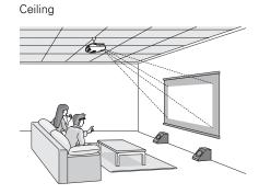
Keep the projector level and place it at a height where its lens is centered between the top and bottom of the screen. If this isn't possible, use the horizontal keystone slider and vertical keystone buttons to adjust the image (see page 21).
