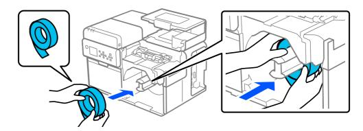
Attach the roll paper flange to the spindle while squeezing the levers of the flange. Move the flange until it touches the roll paper so that there is no gap in between.
