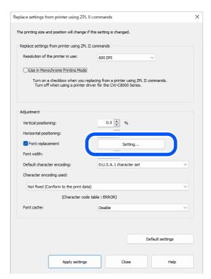
Select the font on the ZPL II compatible monochrome printer to be replaced by specifying the ID of the font.
