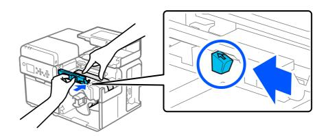
12 Insert the leading edge of the paper into the slot until the paper is automatically fed into the printer.
