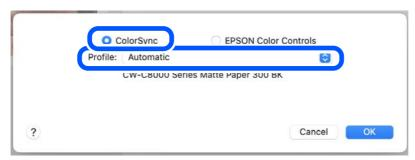
The default profile setting is [Automatic] which automatically selects an ICC profile provided by Epson. Select [Other Profiles...] to display the ColorSync profile selection screen and select a target ICC profile by yourself.
