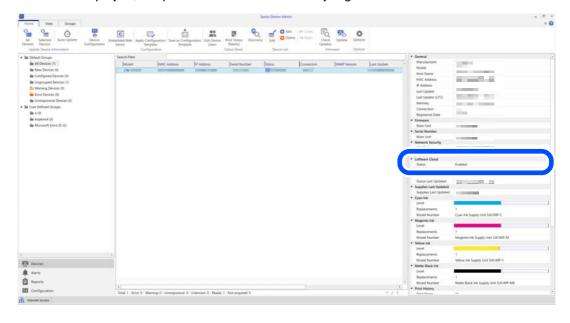
• If "Disabled" or an error number is displayed, the printer registration has failed. Check the solutions listed in "Error Number List" on page 268.
