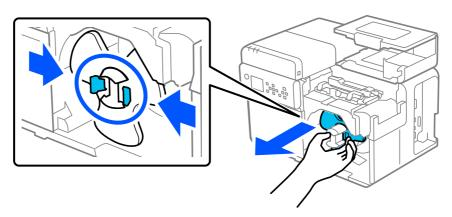
**5** Remove the roll paper from the spindle.
