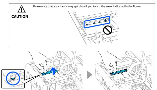
Raise the paper feed slot cover with your finger placed on the tab (shown inside the circle below) and confirm that no labels is stuck to the paper feed slot cover.
