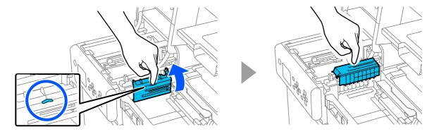
Remove any ink, paper dust, or sticky material adhering to the transparent plate of the gap detector (light emitting side) with a cotton swab moistened with water.
