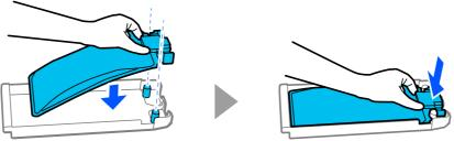
Hold the ink pack tray with both hands and shake it up and down at an angle of about 60 degrees about 10 times in 10 seconds.
