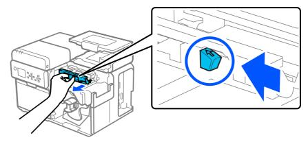
Place the paper in the paper path along the edge guide and align the leading edge with the \_\_\_ mark.
