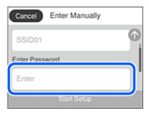
If you enter the SSID manually, set [Password] to [Available], select [Enter Password], and then press the OK button.
