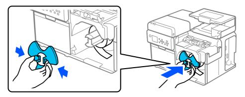
Turn the flange clockwise until the leading edge of the paper touches the bottom, and pull out the paper by approximately 300 mm {11.81 in.}.
