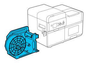
Insert the coupling gear of the rewinder into the rewinder connection opening of the printer. Insert the gear straight against the opening.
