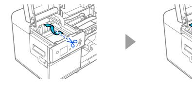
10 Wind up the paper by turning the roll paper flange clockwise until the leading edge of the paper passes through the paper feed slot.
