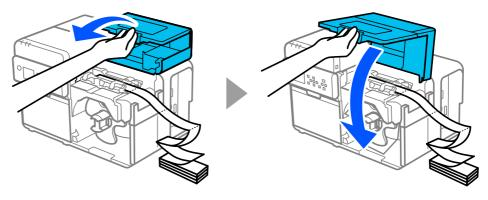
1 1 Place the stack of fanfold paper at least 15 mm {0.59 in.} away from the printer. Be sure that the paper is fed in a straight line to the paper feed slot.
