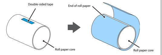
Decide the position and length of the double-sided tape to be applied so that the following conditions are met
