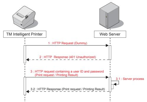
For Digest access authentication, the printer sends a dummy HTTP request before sending a print-related request to the server. The server returns a response with HTTP status code "401 Unauthorized". The printer sends a print-related request containing the user ID and password. The server carries out the Digest access authentication process. Once authenticated, the server continues to carry out the print-related process.
