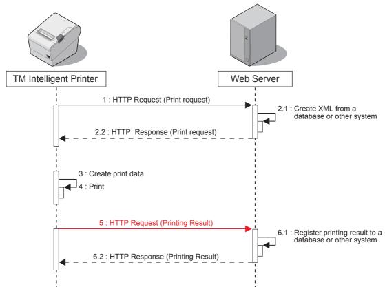
The application can check the printing result (if printing is properly finished) and the printer status by analyzing request data.
