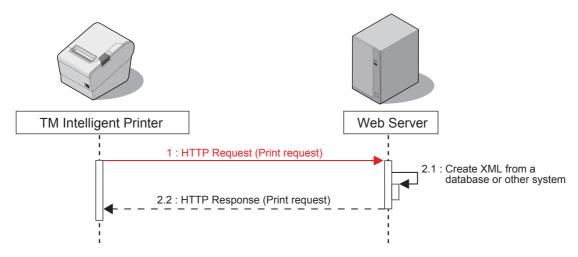
TM intelligent printer periodically sends a HTTP POST request (print request) shown below. The format of request message is URL-encoded form data (application/x-www-form-urlencoded). Set the sending destination and sending interval according to "Server Direct Print Settings" (p. 26). If communication fails, it is attempted again after a specified interval.
