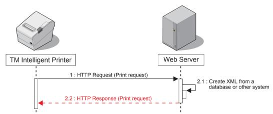
Response data created in XML(text/xml) from the application is returned. The data also contains print data. When an invalid print request is received, the server retries a request (print request) after a specified interval.
