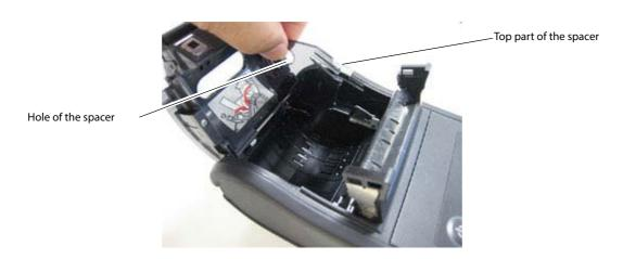
Move the spacer to the position matching the width of the paper you are using.
