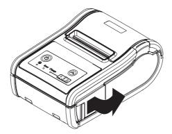
3 Install the battery, and close the battery cover.
