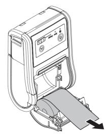
5 Align the left edge of the roll paper with the edge of the cover.
