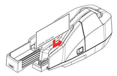
2 After the document is automatically ejected to the Main/Sub pocket, put the next document into the SF.
