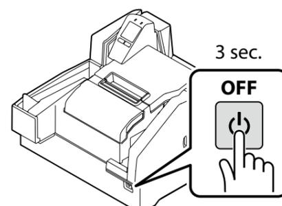
The default connection mode is network. Turn off the product and then change the mode to USB using the switch on the back.
