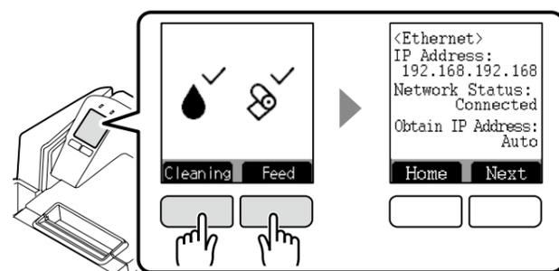
Press the two buttons simultaneously for 2 seconds to display the settings on the screen.
