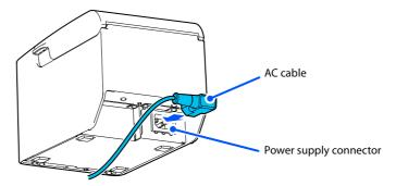
Insert the AC plug into a wall socket.
