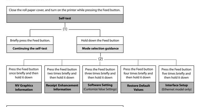
Open the roll paper cover, turn on the printer while pressing the Feed button, and then close the roll paper cover.
