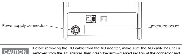
removed from the AC adapter, then grasp the arrow-marked section of the connector and pull straight out.
