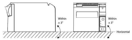
If the printer installation does not fit within the specifications shown in the figure below, the following problems may occur.
