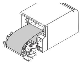
4 Pull out some roll paper, and make sure that the roll paper is set between the paper guides.
