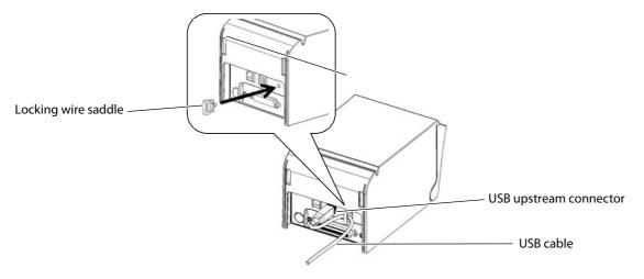
**2** Connect the USB cable from the host computer to the USB upstream connector.
