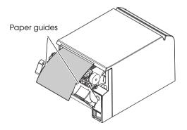
5. Close the printer, and make sure that the roll paper is properly installed between the paper guides.
