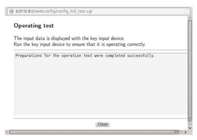
Use the key input device, and check if the registered key input device operates properly.
