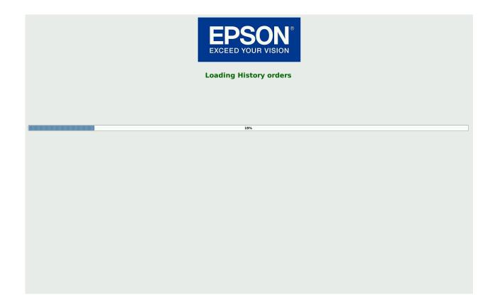
Solution: There is a known issue as of KDS v2.20 caused by invalid network settings for that particular station. Please check the network parameters: IP Address, Mask, and Gateway. Ensure that they are all set properly. If using DHCP, ensure that that the settings are being provided properly by the DHCP server and that the KDS is properly connected to the network.
