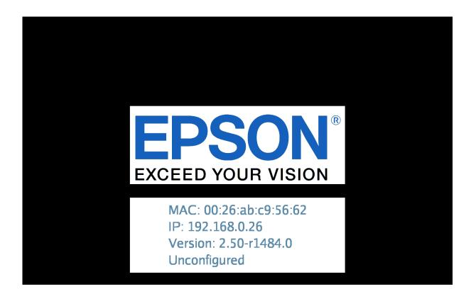
Solution: The KDS needs to be configured using the KDS Configuration Utility.
