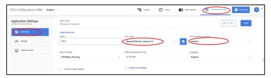
**IMPORTANT:** The POS parser gets installed on the selected POS Connected device and is different for each hardware model. By default, every device ships with a full list of parsers built for itself. The parser name and corresponding IPK filename have the hardware variant in them. For example, in the above picture the POS Type "EpsonKDSmtmc Version 3.4" contains "mtmc", which means MicroTouch Mach platform. Below is the list of supported hardware platforms for each hardware variant.
