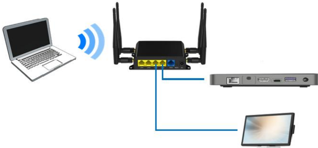
Figure 2.3.1.1: A typical 2 station KDS with a configuration PC or Tablet
