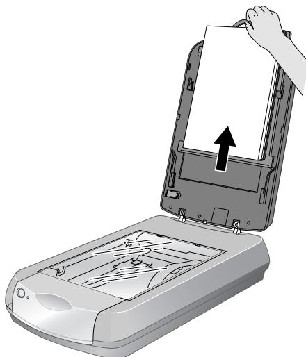
3. If you are scanning film or negatives, open the cover, then slide the film into the corresponding holder, with the film's base side facing down. (If you are scanning slides, go to step 6.)
