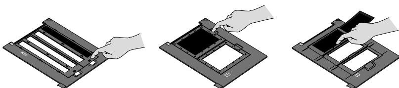
5. Place the film holder on the scanner as shown. Make sure the white triangle on the holder points to the upper-right corner of the scanner.
