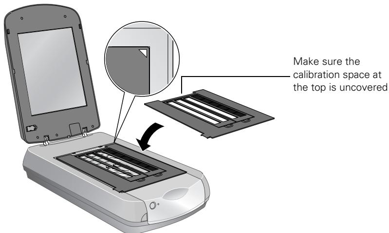
6. If you are scanning slides, place the holder on the scanner. Then place the slides in the holder.
