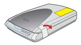
Slide the transportation lock to the unlock position.
